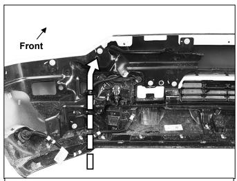
(Fig 1) From below/behind bumper, remove the top outer bumper bracket bolt (arrow) from the back of the bumper. Bumper pictured removed for instruction purposes only, do not remove bumper
