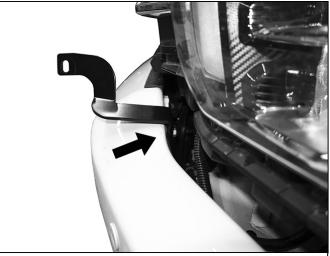
(Fig 4) From behind bumper, reuse bumper bolt to attach driver/left Top Bracket to back of bumper bracket (arrow). Bumper pictured with top fascia body panel removed for instruction purposes only, do not remove fascia panel
