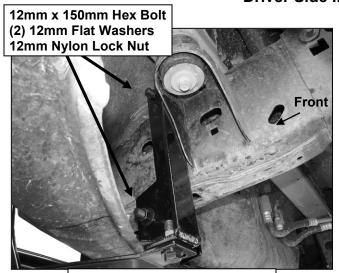
(Fig 10) Outer Support Bracket
