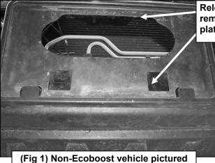
Release clips to remove license plate bracket
