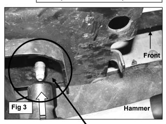
Remove factory hex nut. Drive bumper bolt back through hole with hammer to break tin retaining clip. IMPORTANT: Do not damage threads on bumper bolt!
