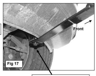
12mm x 40mm Hex Bolt (2) 12mm Flat Washers 12mm Lock Washer 12mm Hex Nut
