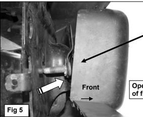
Hold the bumper bolt out of the way and insert Frame Bracket between bumper cover and bumper bracket. Line up hole in Bracket with bumper bracket and reinsert bumper bolt
