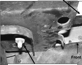
(Fig 2A) Remove factory hex nut (Driver side, non Ecoboost vehicle pictured from behind bumper)
