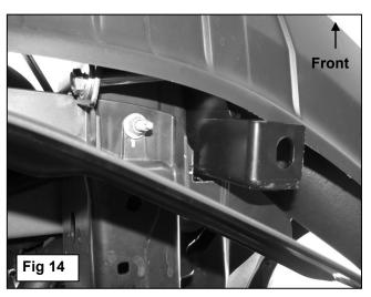
Factory air dam mounts to each frame rail in this location.
