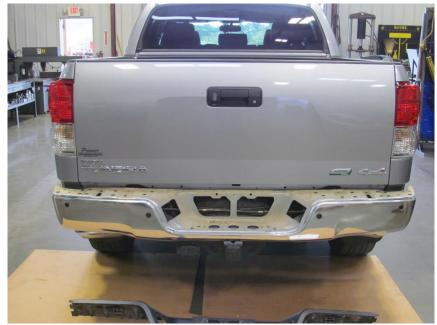
8. Using 12mm socket/wrench remove six bolts located on top of chrome OE bumper top surface.
