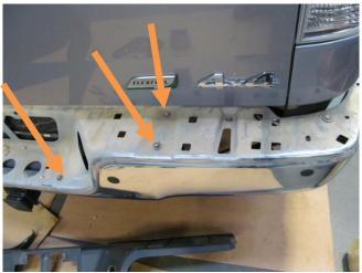
9. Use 12mm socket/wrench to remove two bolts located underneath of bumper (one on each side). See Figure 10.
