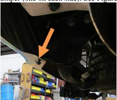
10. Using a 19mm socket remove three bolts from receiver hitch. (Both sides)
