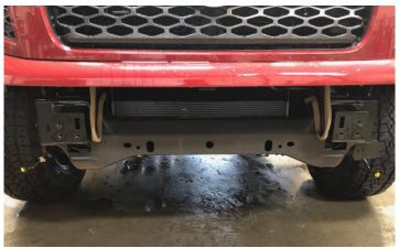
8. Remove the sensors, grommets, and sensor wiring harness from the OE bumper. **Be sure to note the position of the grommets, so that they can be installed in the correct locations on your new Hammerhead bumper.**
