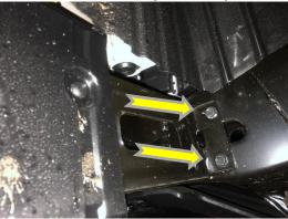
4. Remove the plastic covers around the tow hooks by pulling away from the front of the vehicle. Disconnect the sensor (if applicable). NOTE: When removing the covers be mindful of the sensor wiring harness so that you don't break the harness.
