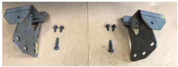
4. Using a 14 mm socket or wrench, a 17 mm socket or wrench, and hardware from hardware kit #188, attach the frame mounts to the frame of the truck. Use 4 washers on each of the bottom mounted OE bolts. Do not fully tighten.
