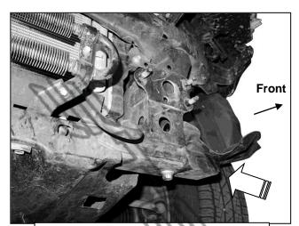
(Fig 6) Remove aluminum inner bumper from frame. Also remove outer frame ends from crossmember, (arrow).
