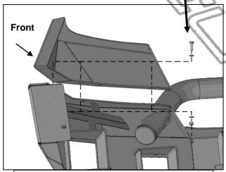
(Fig 12) Attach Fill Panel to top of Bumper
