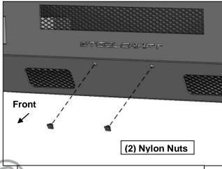
(Fig 15) Attach License Plate to Bumper
