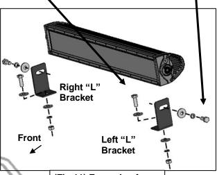
(Fig 11) Example of center light installation
