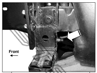
(Fig 10) Insert 12mm x 120mm Hex Bolt through Bracket and cross member
