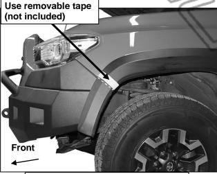
(Fig 16) Cut front end off of the fender flare to match up to Bumper
