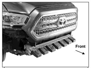
(Fig 5) Remove plastic impact bumper and aluminum crossbar from bumper brackets
