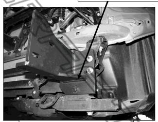
(Fig 9) Driver/left Mounting Bracket attached to end of frame
