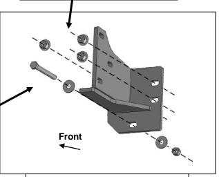
(Fig 7) Attach driver/left Mounting Bracket to end of frame
