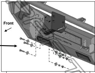
(Fig 13) Attach Bumper to Frame Brackets
