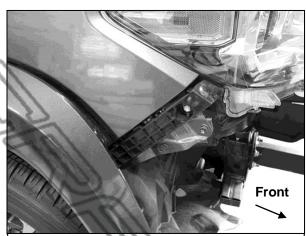
(Fig 4) Remove plastic block (arrow) from front edge of fender. Reinstall hardware to secure headlight
