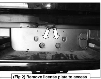
(Fig 2) Remove license plate to access and remove (2) hex bolts (arrows)
