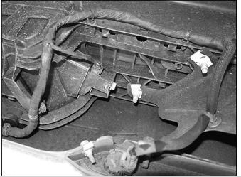
(Fig 5) Remove license plate lights, remote antenna (Fig 10), parking sensors and wiring harness
