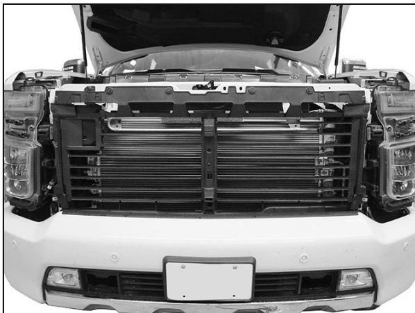
(Fig 7) Grille and fascia removed
