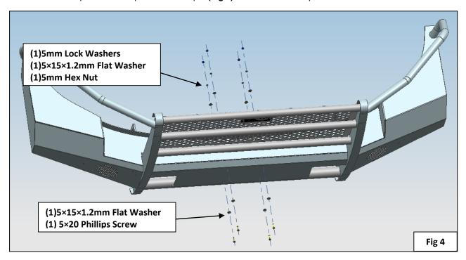
Install the Brackets(left and right) and the Bumper to the frame. Fasten the Brackets and the Bumper with the hardware (Fig 5).
