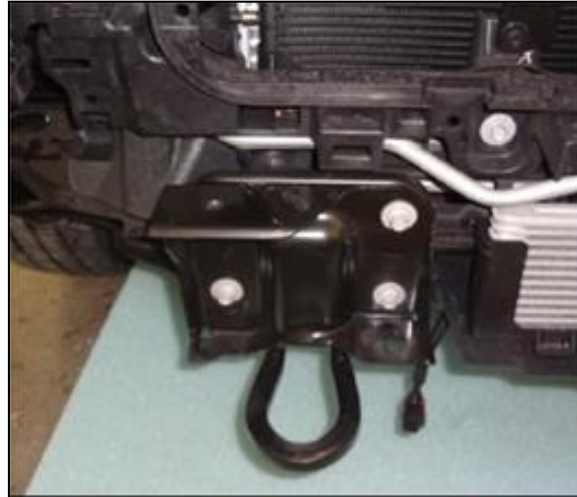
Figure 3b (Tow Hook & OEM Mounting Bracket)
