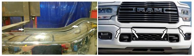
2. If tow hooks are not present, cut out the plastic around the two locations where tow hooks would be *(see photo below)*. If present, remove the factory tow hooks to insert the bottom brackets. Note: Some trimming to the plastic around the tow hook may be required.
