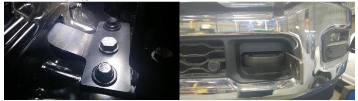
4. Install top mounting bracket. The bracket will be installed from the bottom side of the truck. Remove the top nut of the bumper bracket. Slide the flat side of the top bracket through the opening of the bumper and grille. (1<sup>st</sup> Photo is shown from looking up from under the truck. 2<sup>nd</sup> photo (passenger side) shown with bumper off for location purposes.)
