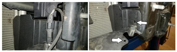
8. Unbolt the bumper by removing the (2) 8mm bolts, *one on each side*, front splash guard bolts and (6) 21mm bumper nuts, *three on each side*.
