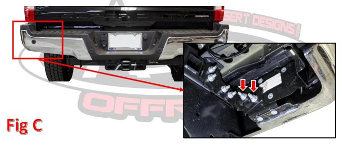
4. Remove the OEM Bumper Mounting Brackets. Use a 21mm Socket to remove the four mounting bolts (per side), then remove the bracket. Save these bolts for reuse. (Fig D)
