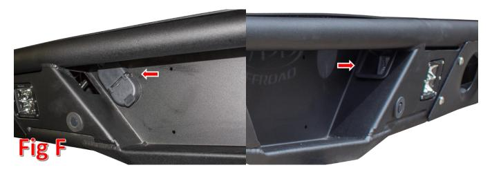
4. Push the parking sensor mounting rings into their precut holes on your new bumper. If the mounting rings do not click into place you may have to trim the mounting tabs slightly. Make sure to install these in the same position and order as they came off your OEM bumper. Refer to Fig G.
