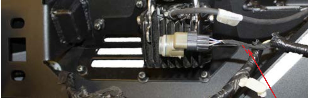
Cut sensor wires here
