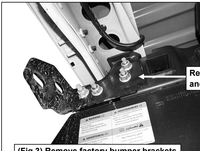
(Fig 3) Remove factory bumper brackets
