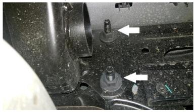
7. Lastly, remove the two 13mm bolts that are located behind the license plate and remove bumper.
