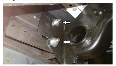
11. Mount the factory side bumper bracket to the tab located under the enc cap. Use 5/16" hardware.
