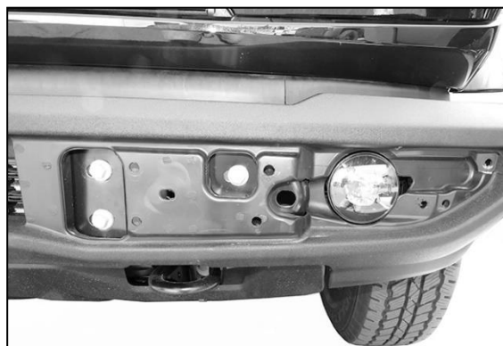
(Fig 2) Models with plastic bumper cover (see Fig 1), remove bumper pads from bumper (driver/left side pictured)
