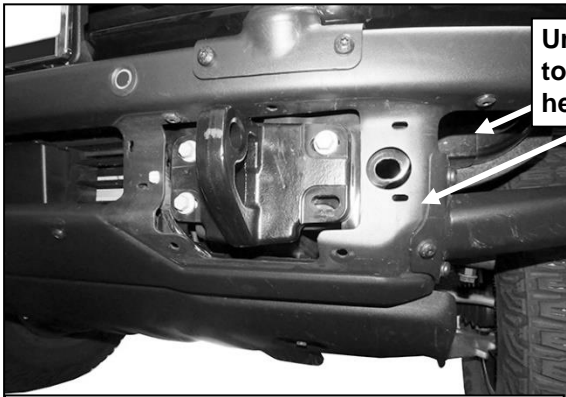
(Fig 3) Model with steel bumper, remove cover from bumper (driver/left side pictured)
