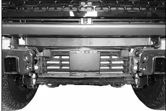
(Fig 4) Remove factory hex bolts from front to remove bumper assembly
