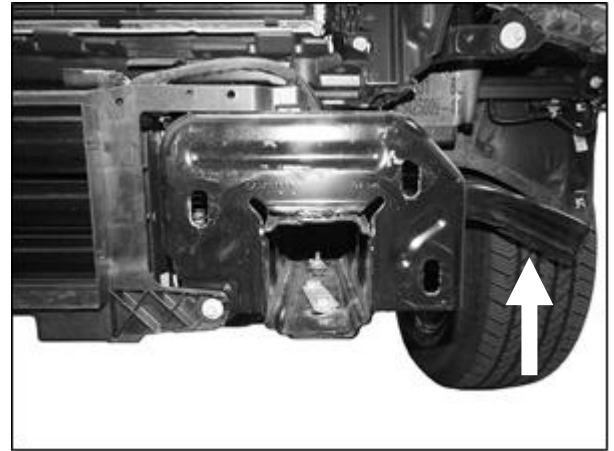
(Fig 6) Remove bumper. Also remove the factory frame extension (arrow-optional)
