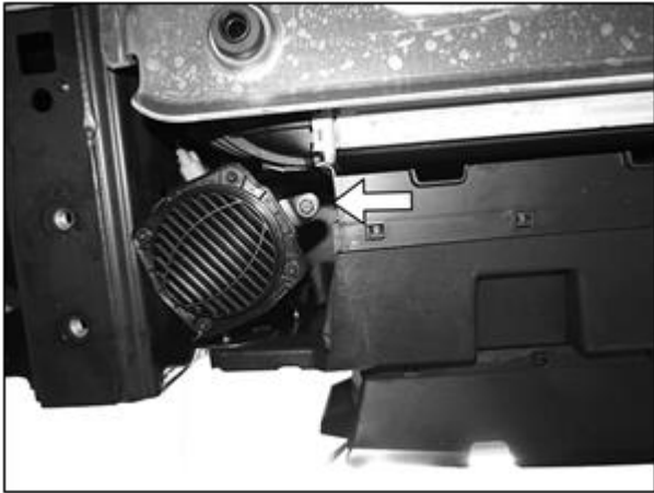
(Fig 5) Remove bolt (arrow) to temporarily remove audible alert speaker located behind driver/left side of bumper (hybrid models only-pictured from below)
