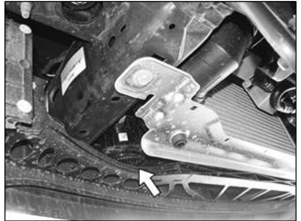
(Fig 4) Hybrid Models Only, locate alert speaker behind driver/left side of bumper
