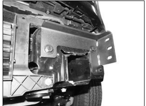
(Fig 8) Driver/left side Bracket installed
