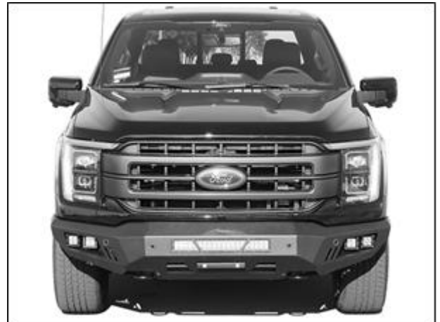
(Fig 15) Attach Bumper to Frame Mounting Bracket (passenger/right side illustrated)
