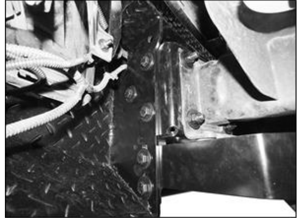
(Fig 16) Driver/left side of Bumper and Support Bracket installed
