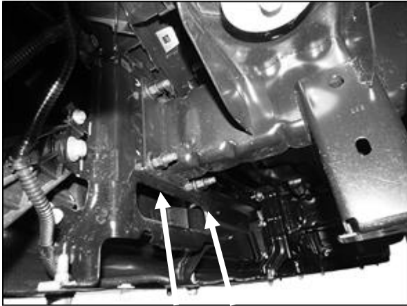
(Fig 5) Remove (3) factory hex nuts from each side (back of bumper pictured from below)
