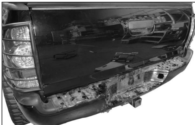
(Fig 3) Models with receiver hitch only, remove plastic cover from top of bumper to access hex bolts attaching bumper to top of receiver hitch
