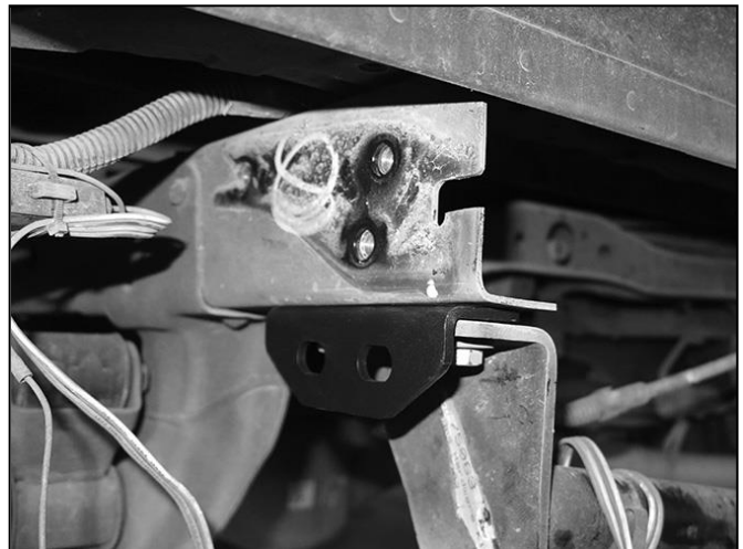
(Fig 7) Attach Support Brackets to bottom of frame. On models with aftermarket hitch, insert Bracket between bottom of frame and hitch
