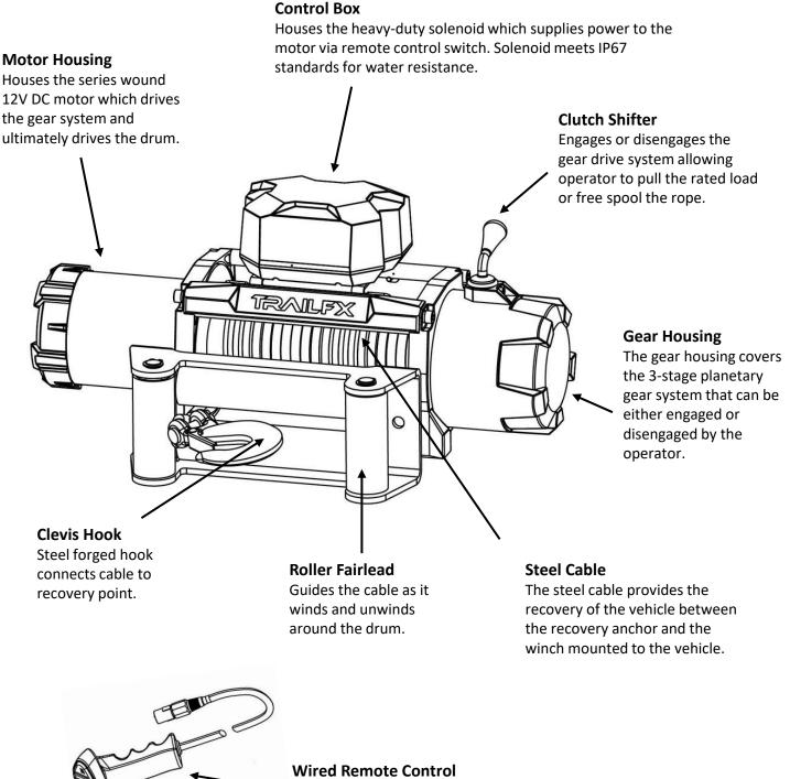
Allows the operator to control the winch from a safe distance.
