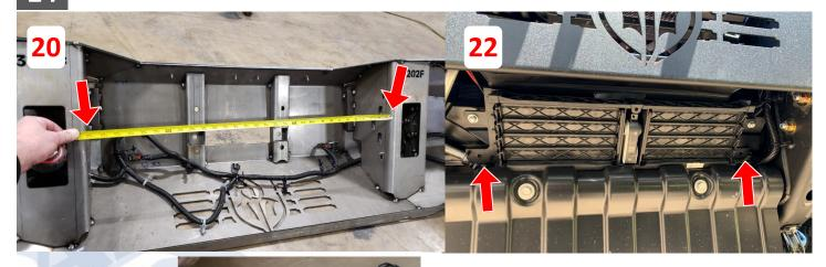
Install the winch to the bumper using the supplied Allen Bolts and Washers.
