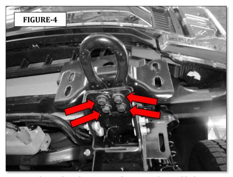
**Step-7** Using an 18mm socket and ratchet remove the nuts and paired bolts securing the under rider guards to the frame rails, (FIGURE 5). Retain the nuts and paired bolts as they will be used for installation of the frame brackets.
