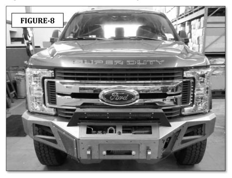
**Step-9** Re-install the passenger and driver side front vent covers to the bumper shell using the  $\frac{1}{4}$ " x 1" button head bolts,  $\frac{1}{4}$ " plastic flat washers and  $\frac{1}{4}$ " rubber rivet-nuts removed in step 4, (FIGURE 9).
