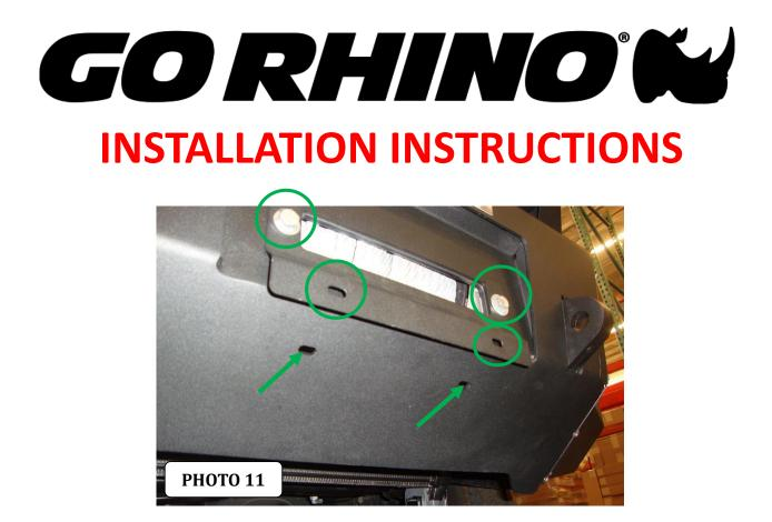
If installing a winch, attach the license plate directly to the (2) obround holes in the lower face of the bumper shell using the supplied  $\frac{1}{4}$ " bolts and nuts.
