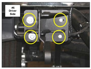
**Step-10** With assistance attach the bumper shell brackets to each frame bracket using (2)  $\frac{1}{2}$ " x 1  $\frac{1}{2}$ " hex bolts, (4)  $\frac{1}{2}$ " flat washers, (2)  $\frac{1}{2}$ " lock washers and (2)  $\frac{1}{2}$ " Hex nuts, Align the bumper shell with the vehicle, verify that the tailgate clears when lowered, and tighten all nuts and bolts, (Photo 7). If necessary loosen the frame / receiver hitch bolts to adjust the bumper shell.
