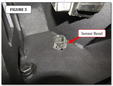
**Step-4** Transfer the wiring harness for the parking sensor/license plate lights to the bumper replacement. Install the parking sensors into each bezel, making sure to install the sensors in the same order as they were removed from the OEM bumper. Install the license plate lights into the housings, (FIGURE 4).
