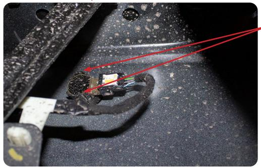
SPREAD THESE TWO TABS - TO RELEASE THE PARKING Sensor.
