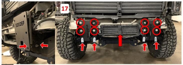
Install all sensor into Evolution bumper as were in factory bumper. Trim 1/16" off sensor housing for proper fit. Zip tie can be used on back side to secure each sensor assembly to bumper.
