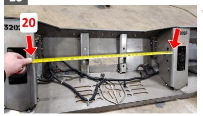
\*MINIMUM 3/8"+ Gap Required; DO NOT Install
