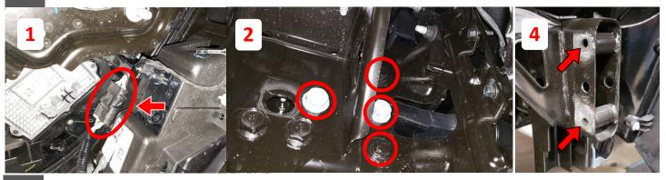
Loosen two bolts securing each intercooler bracket to inside of frame. (Do not remove from frame) 5 6 Loosely install frame crush brackets followed by given 1/2" x 4" bolts through frame end . (Hook end first) 7 Replace factory nut plate with given 1/2" hex nuts, washer, and lock washer 8 Install each frame bracket using OEM bolts, washers & nuts; followed by given 1/2" x4" bolts.
