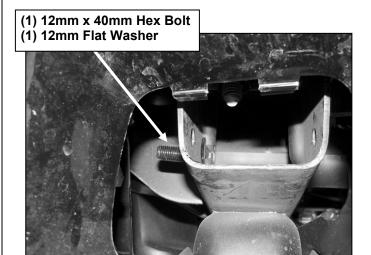
(Fig 3) Passenger side frame channel pictured
