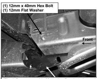
(Fig 4) Passenger side Mounting Bracket pictured
