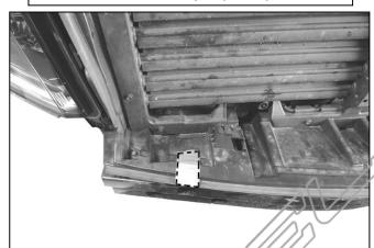
(Fig 7) Passenger side approximate cut out on Plastic cover to clear Bracket
