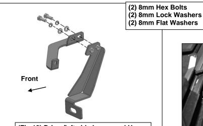
(Fig 18) Driver/left side Lower and Upper Bracket Assembled above
