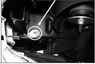
(Fig 16B) Driver side Bracket installation pictured without plastic panel for instruction purposes only
