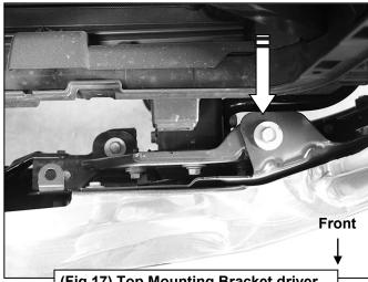
(Fig 17) Top Mounting Bracket driver side mounting location from above
