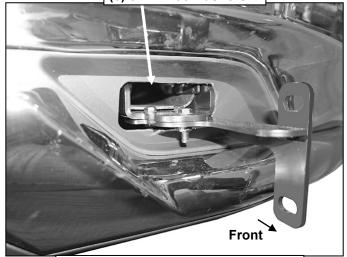
(Fig 16) Driver side Bracket Installed
