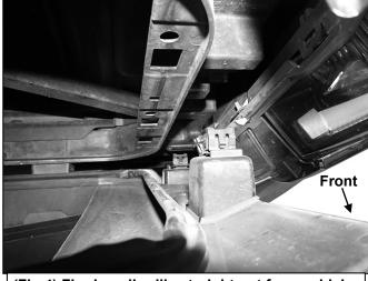
(Fig 4) Firmly pull grille straight out from vehicle
