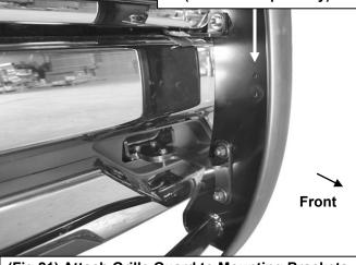
(Fig 21) Attach Grille Guard to Mounting Brackets
