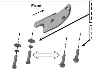
(2) 12-1.25mm x 55mm Fine Thread Hex Bolts (2) 12mm Lock Washers (2) 12mm Flat Washers
