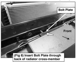
**Top Support Brackets attach to holes** (arrows) in radiator cross-member (see Fig 8)
