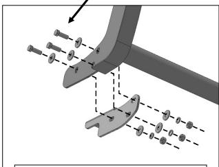
(Fig 11) Attach Grille Guard to Frame Brackets (passenger/right side illustrated)
