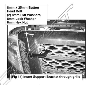
8mm x 25mm Button Head Bolt (2) 8mm Flat Washers 8mm Lock Washer 8mm Hex Nut
