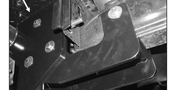
(Fig 15) Driver/left side of Bumper attached to Bracket assembly, (pictured from behind Bumper)
