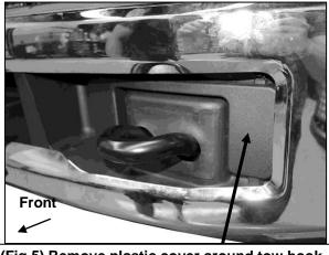
(Fig 5) Remove plastic cover around tow hook
