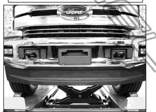
(Fig 3) Remove plastic air dam from bumper
