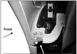
(Fig 2b) Pull back fender liner to locate fascia attachment at bottom of front fender
