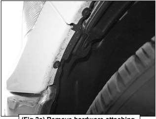
(Fig 2a) Remove hardware attaching plastic fender liner to fender
