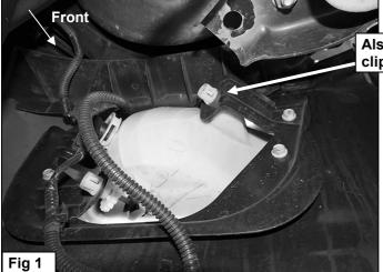
Also release all wiring clips from bumper
