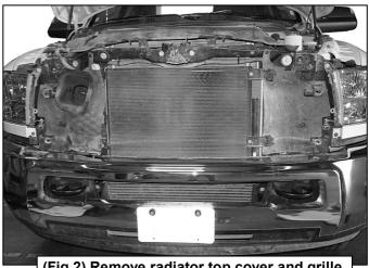
(Fig 2) Remove radiator top cover and grille
