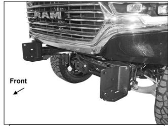
(Fig 8) Frame and Support Brackets installed
