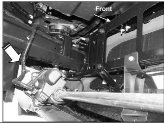
(Fig 2) Remove hex nuts attaching bumper. Temporarily remove active air dam for better access to bumper hardware. Back of bumper pictured
