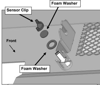
(Fig 12) Slide sensor into sleeve, insert Foam Washer and Clip to lock sensor in sleeve
