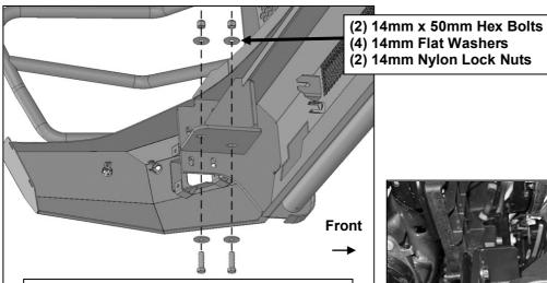
(Fig 15) Attach driver/left tow hook to Bumper
