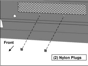
(Fig 21) Attach License Plate Plugs to Bumper
