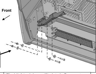
(Fig 14) Attach lower (2) slots in Bumper to inside of Frame Bracket and Support Bracket
