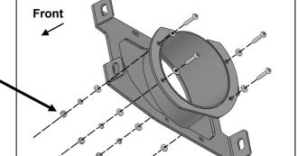
(Fig 18) For models equipped with round fog lights, use the Round Light Brackets
