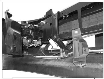
(Fig 10) Remove sensors, harness and fog lights as equipped from factory
