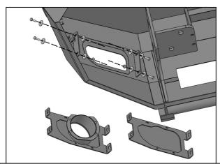
(Fig 19) Reuse the hardware from the square light bracket. For models with round fog lights, attach the Round Light Bracket to the back of the bumper. For models without fog lights, attach the Cover Panel to the back of the bumper
