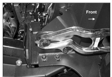
(Fig 16) Tow hook installed
