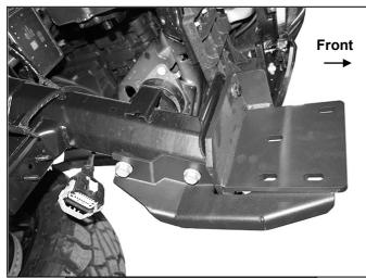
(Fig 7) Driver/left Support Bracket attached to bottom of frame
