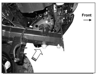
(Fig 4) IMPORTANT: Loosen but do not remove rear bolt (arrow). Driver/left side pictured
