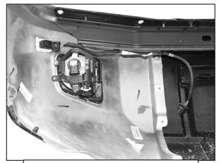
(Fig 16) Remove sensor and fog light
