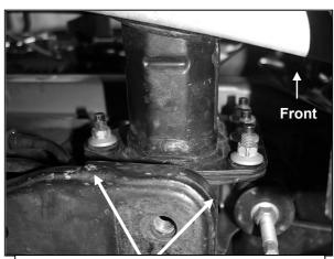
(Fig 9) Remove hex nuts attaching bumper brackets to end of frame. Driver/left side bumper bracket pictured from below
