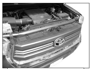
(Fig 1) Remove plastic cover and grille
