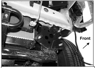
(Fig 10) Bumper removed, driver/left pictured
