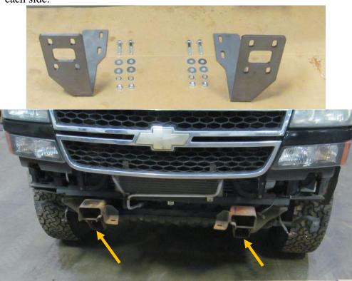
4. Using a hoist or a few friends, attach bumper to frame mounts using hardware kit #0001 Start all bolts before aligning bumper. Align bumper a minimum of ½" below headlights. When truck flexes off-road, this distance allows your bumper and body to have clearance. Tighten bolts with ¾" socket and wrench. Tighten frame mount bolts at this time.
