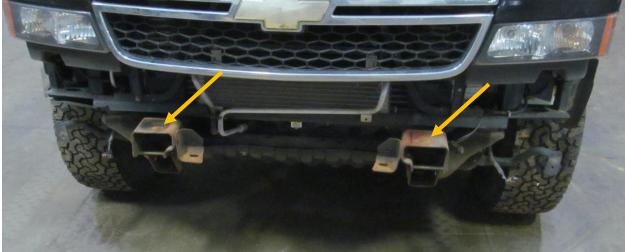
3. Install lower mounts (0932 &0933) on bottom of frame. Use one hardware kit # 0004 on each side.
