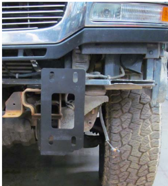
FIGURE 15: FRONT VIEW OF FRAME MOUNT
