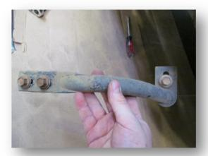
3. Using a 21mm socket remove two nuts from the bolt strip holding the bumper to the frame of vehicle. (Both sides)
