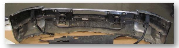
6. Using 18mm socket and wrench remove the single bolt holding on the OEM tow hook (both sides).
