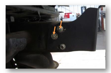
3. Using an 18 mm socket and 18mm wrench tighten tow hook bolt and nut.
