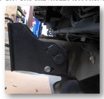
Figure 10: Outside side view of driver side frame mount
