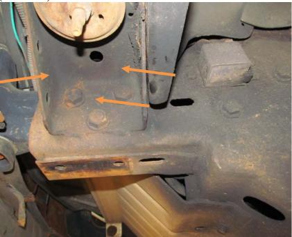
3. Pull bumper out two inches. Using 18mm socket remove bolts on top and bottom of side brace. Set brace aside. (both sides) Set OEM bumper aside.
