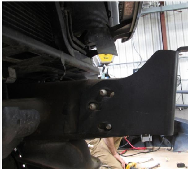
Figure 11: Inside side view of driver side frame mount
