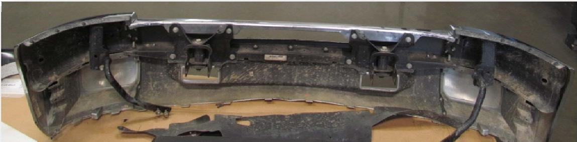
6. Using 18mm socket and wrench remove the single bolt holding on the OEM tow hook (both sides).
