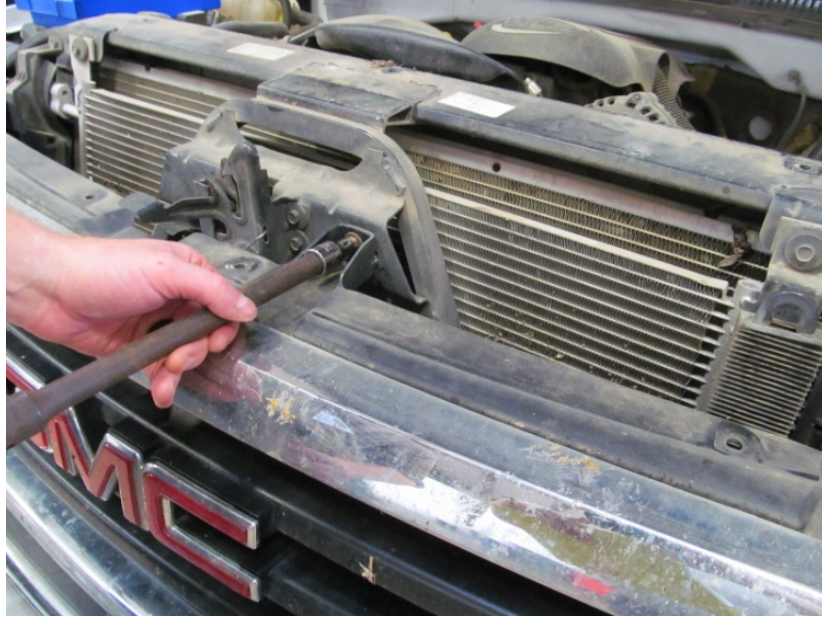
FIGURE 2. REMOVAL OF TOP GRILL BOLT
