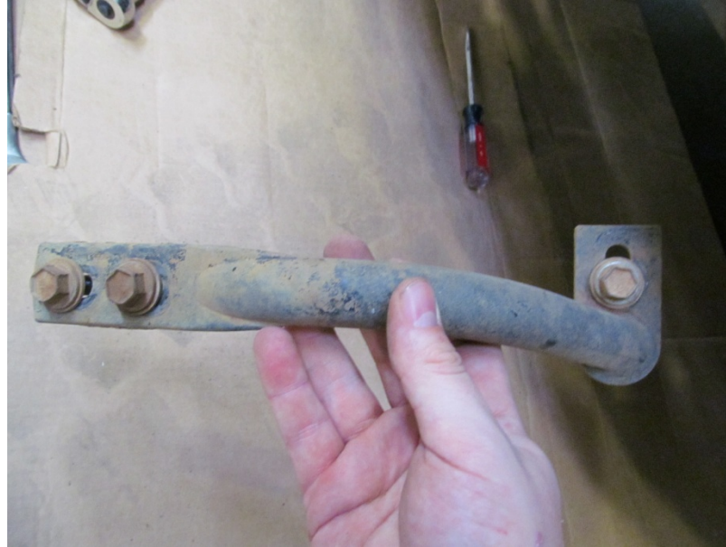
FIGURE 8: OUTSIDE BRACE REMOVED FROM FRAME
