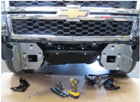
2. Install Hammerhead lower frame mounts (601-56-2154 and 601-56-2156) and loosely tighten. Use OEM hardware for thru frame bolt and use two  $\frac{1}{2}$ "-13 x 2" bolts, four flat washers, two lock washers and two nuts from Hardware kit #1 bolt for the lower bolts. (orange arrow).
