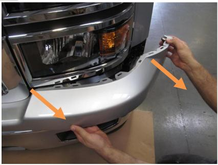
3. Release six tabs on center of plastic trim below the grill. Have a friend gently pull out on the plastic trim as you release the tabs behind the grill. A flathead screwdriver works well to help pry the tabs. Set aside plastic trim.
