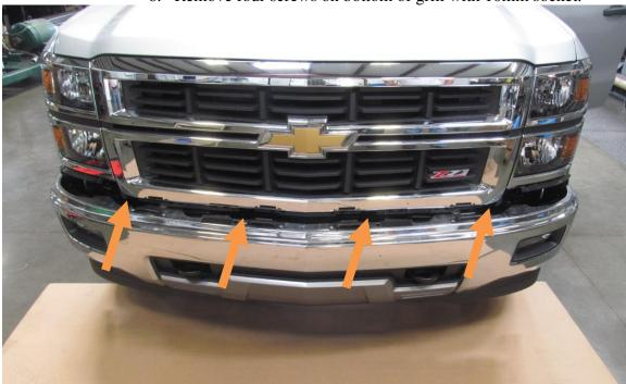
7. Pull up and out (toward your body) on the top of the grill where the screws were to release the plastic tabs. Using your thumbs to push down on the bracket makes it easy.
