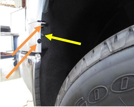
2. Pull out on edge of plastic trim to release the tabs as shown. Pull in direction of arrows. (both sides)
