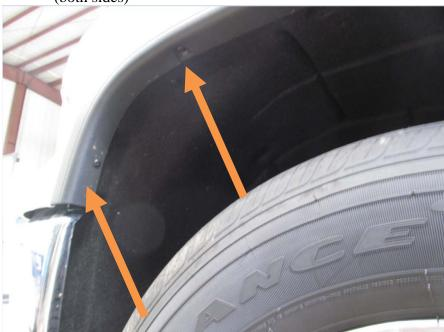
2. Gently pull away from truck on OEM fender flare as shown. (both sides)
