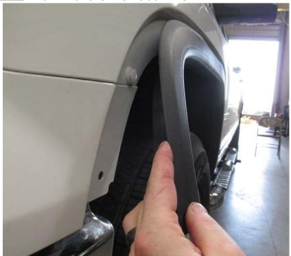
3. Remove screw holding on plastic trim piece with 7mm socket. (both sides)
