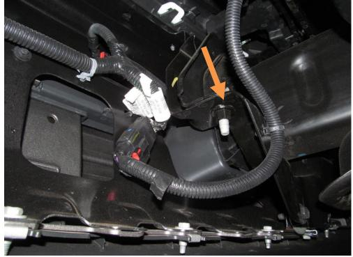
8. Remove three bolts from OEM side bumper support (in front of tires) with 15mm socket. (both sides)
