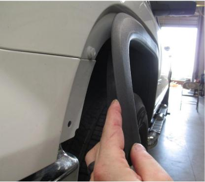
3. Remove screw holding on plastic trim piece with 7mm socket. (both sides)
