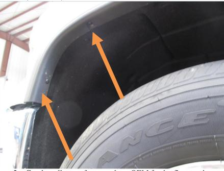
2. Gently pull away from truck on OEM fender flare as shown. (both sides)
