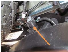
2. Unplug OEM license plate and sensor wiring harnesses
