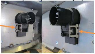
3. Install OEM spare tire access housing.
