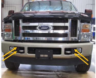
4. Using 16mm socket remove three bolts holding on OEM tow hook and set aside. Access bolt heads from bottom. (both sides)
