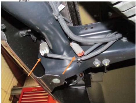
3. Using an 18mm socket, remove lower bolt from receiver hitch. This bolt holds on the lower portion of the OEM bumper shell. (both sides)
