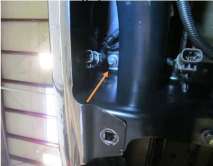
5. Using a 17mm socket, remove two bolts from bottom of receiver hitch. (both sides)
